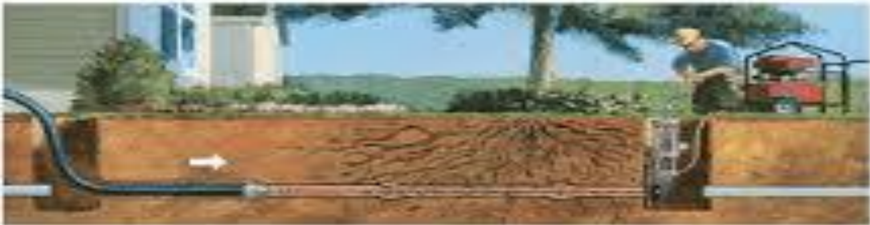
Trenchless Repair Methods
